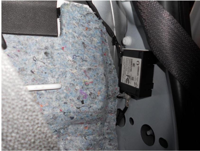
Figure 3 – Original TPMS Receiver Location
