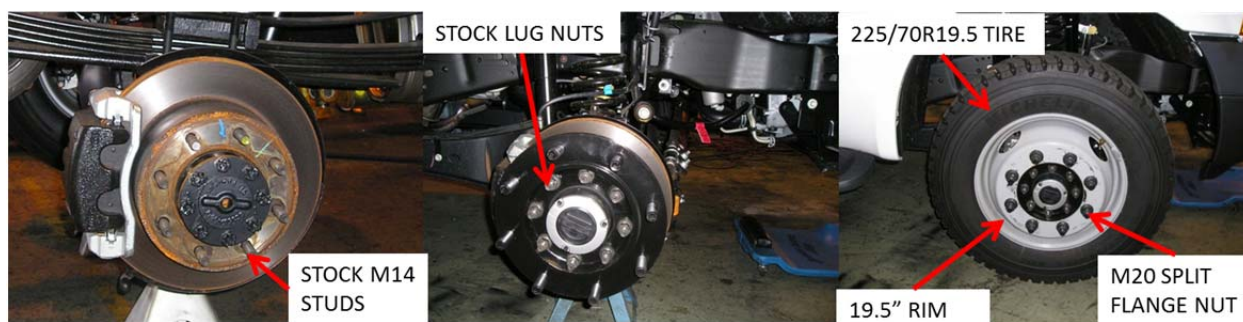
Figure 2 – Wheel Adapter Details
