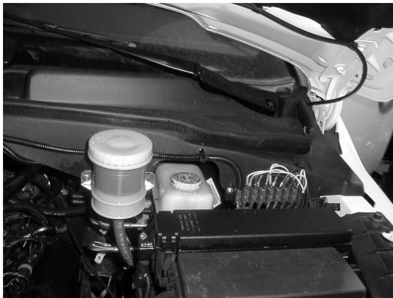
Figure 4.8.3: Typical Reservoir Installation
