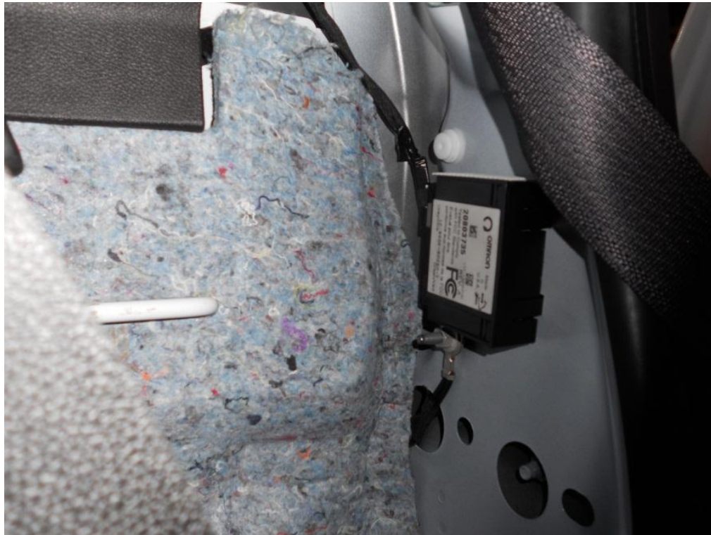
Figure 3 – Original TPMS Receiver Location
