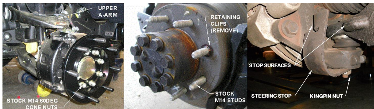
Figure 2 – Wheel Adapter Details
