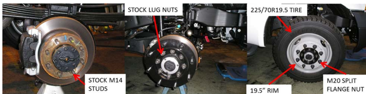
Figure 2 – Wheel Adapter Details
