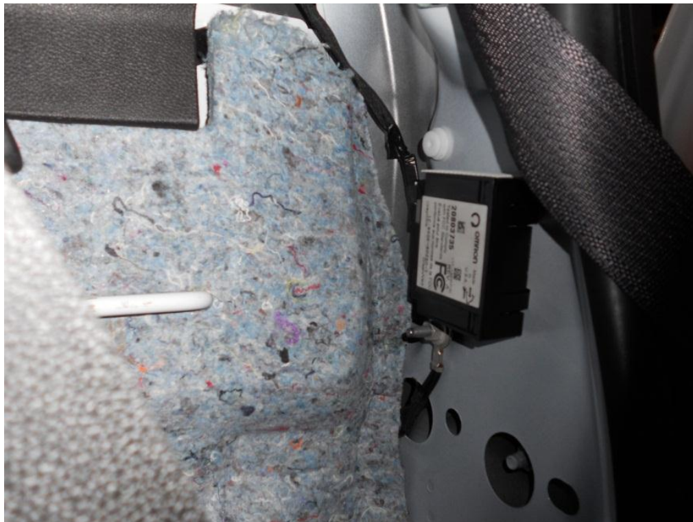
Figure 3 – Original TPMS Receiver Location
