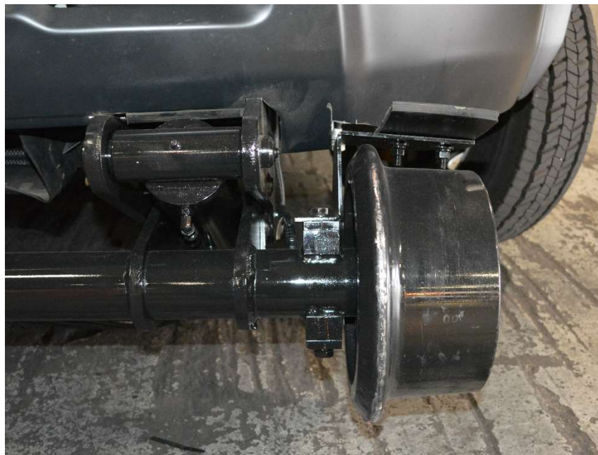
Figure 4.5.4.D '08+ Ram Front Bumper Trimmed
