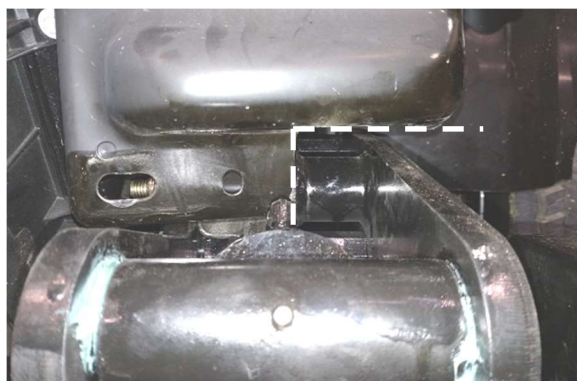
Figure 4.5.4.B Ram Bumper Bracket Modification (DS shown).
