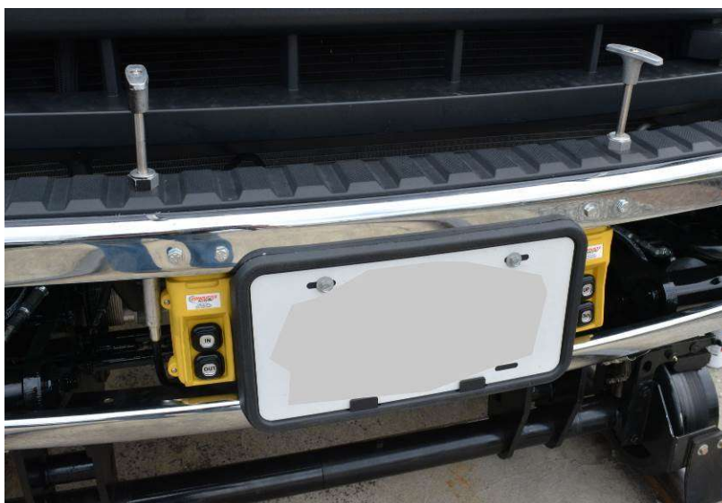
Figure 5.3.2 Typical Front Manual Pin Off Cable Mounting
