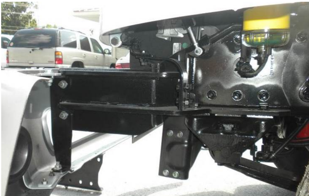
Figure 1. M2 106 with 8" bolt-on frame extension; driver's side
