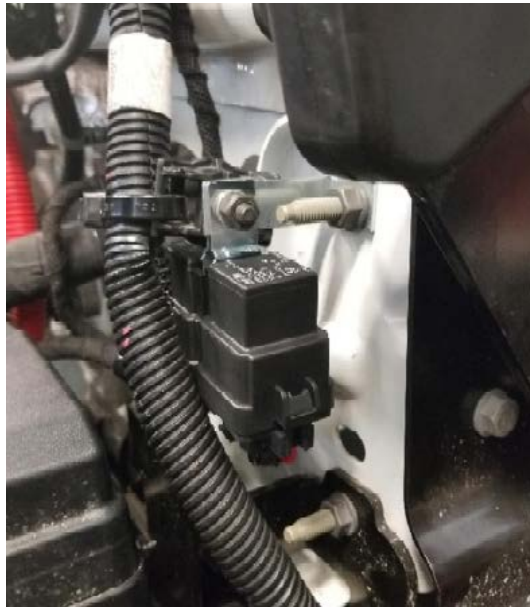
Figure 2. Suggested Relay Mounting Location (Firewall, Driver's Side)
