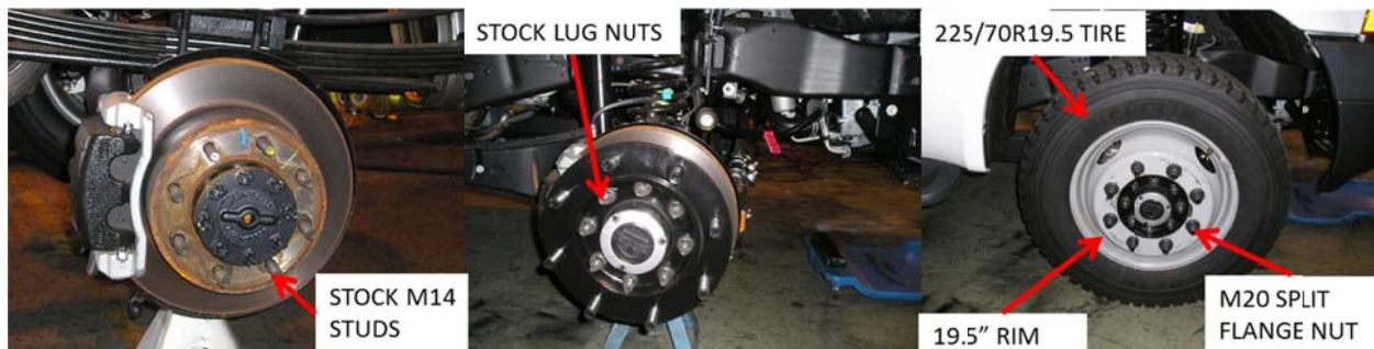
Figure 2 – Wheel Adapter Details
